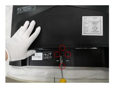
Step.3 Separate hooks between MID\_FRAME and R/C
