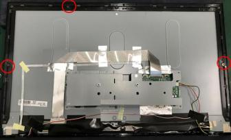
Step10. If with speaker model, assembly speaker on middle frame, and assembly speaker cable on main board. (red and white cable is on left side, yellow and black is on right side.)
