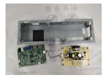
Step.8 Remove connecter cable and separate main board and power board, separate mylar and shielding
