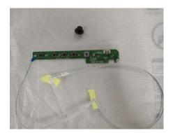
Step.12 Separate wall-mount BKT and display key from rear cover
