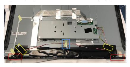
Step12. Insert key board FFC on main board
