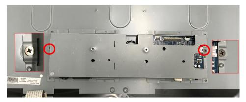
Step4. Use Al tape to fix shielding (tape in blue circle).
