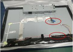
Step.6 separate SPK from MID\_FRAME and LVDS & Backlight FFC from LCM
