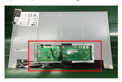
Step2. Insert 30 pin LVDS FFC to LCM,
