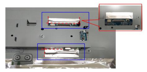
Step5. Insert 10 pin back light FFC to panel and main board, use yellow tape to fix. (Tape in red circle).
